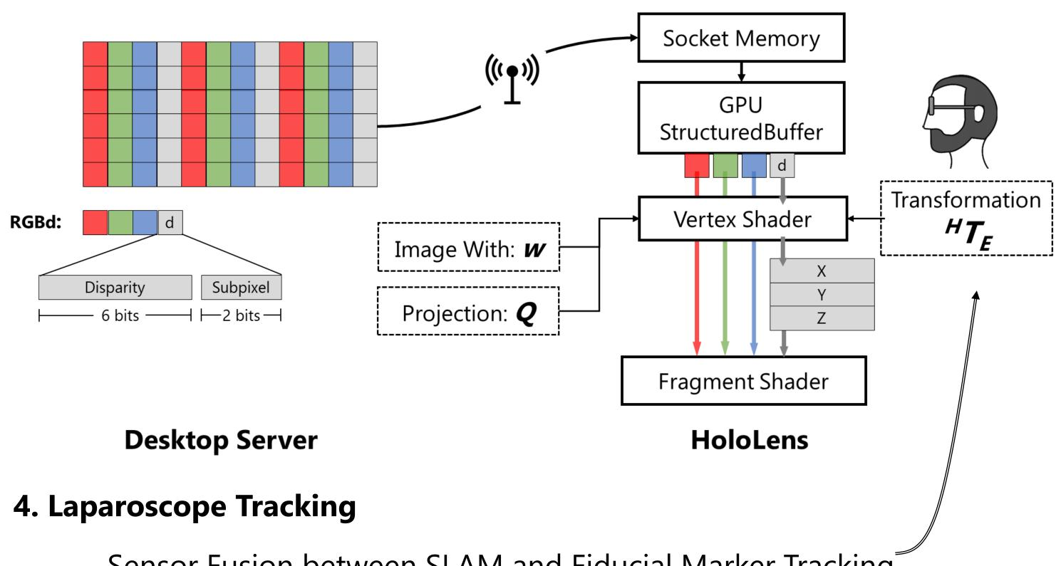
Sensor Fusion between SLAM and Fiducial Marker Tracking
